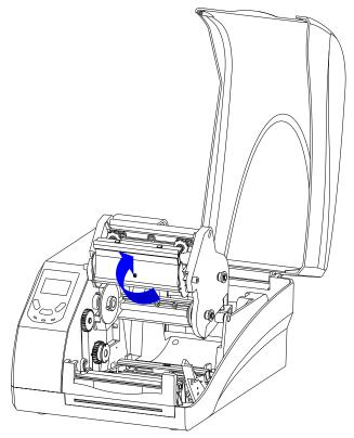
Figure 2-5 Lift the Printhead Module
