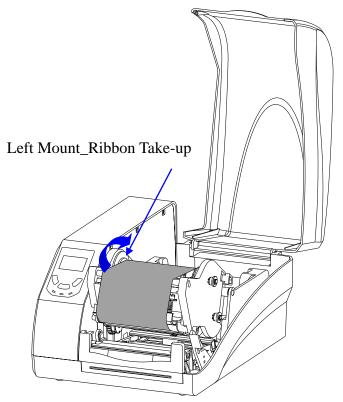
Figure 2-10 Ribbon Roll loaded
