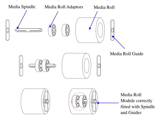
Figure 2-11 Place Media Roll on Media Spindle
