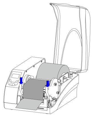
Figure 2-13 Press Down to Lock the Printhead Module
