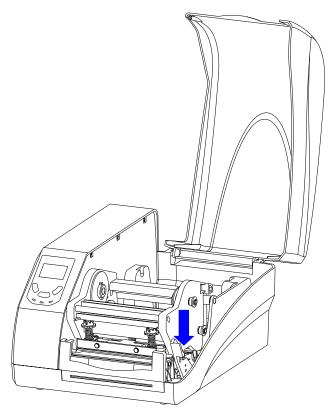
Figure 2-4 Release the Printhead Module
