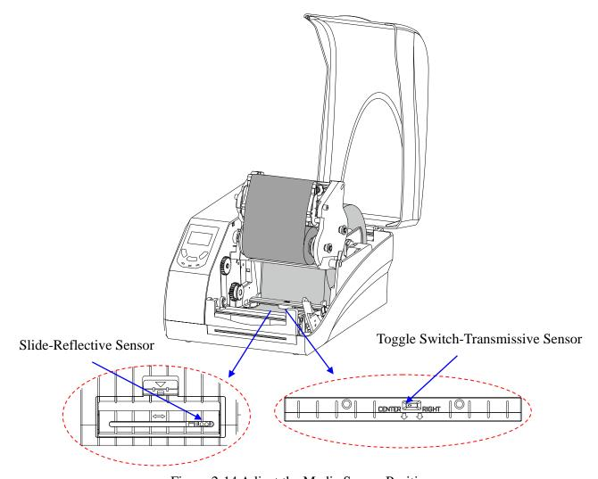
Figure 2-14 Adjust the Media Sensor Position
