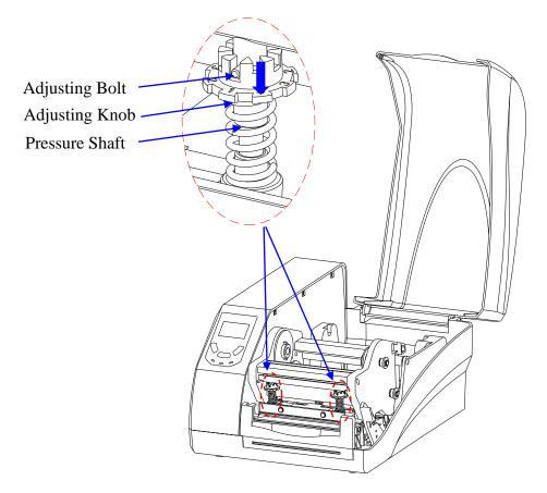
Figure 3-3 Printhead Pressure Adjustment
