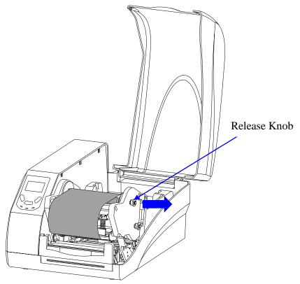
Figure 2-9 Place the Core on Ribbon Take-up
