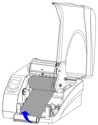
Figure 2-8 Wrap Ribbon on the Core
