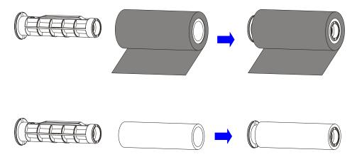
Figure 2-6 Place Ribbon Roll and Spare Core on Ribbon Spindles
