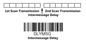
To remove this delay, scan the **Intermessage Delay** bar code, then set the number of delays to **0**. Scan the **Save** bar code from the Programming Chart, beginning on page 253.
