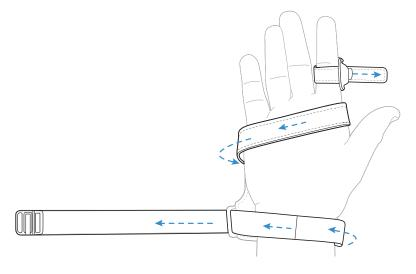
4. Fasten the strap on the index finger. Continue to tighten the strap around the wrist.
