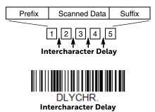
To remove this delay, scan the **Intercharacter Delay** bar code, then set the number of delays to **0**. Scan the **Save** bar code from the Programming Chart, beginning on page 253.
