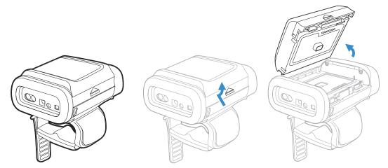
Replace the battery by snapping it in to the 8680i.
