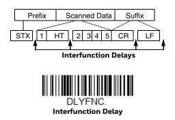
To remove this delay, scan the **Interfunction Delay** bar code, then set the number of delays to **0**. Scan the **Save** bar code from the Programming Chart, beginning on page 253.
