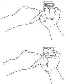
7. Press the trigger to power up the scanner. The battery, WiFi, and Bluetooth status appear in the window.
