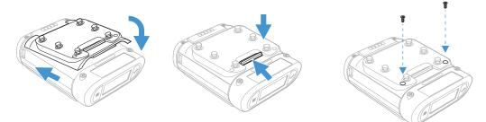
3. Use the 2 screws to secure the glove mount to the 8680i.
