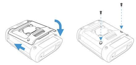
3. Use the 2 screws supplied with the trigger to secure the plate to the 8680i.
